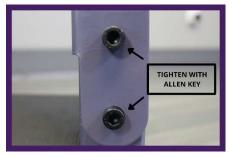
2) Before adjusting the height of the upright arms, be sure to loosen the spring pins by turning them counterclockwise. Adjust the arms to the desired height then tighten the spring pins by turning them clockwise.
